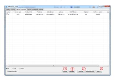
Step 2: For multi-devices batch upgrade, user need to modify the default IP address to different one to avoid IP address collision. Take a example as below pic shows:
